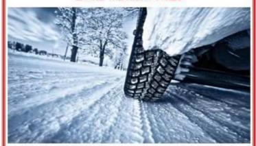
minimum tyre tread 1.6mm although it is advised to have no less that 4mm while driving in winter conditions to maintain optimal grip levels. These tires retain their softness at lower temperatures and therefore provide a stronger grip on slippery surfaces.
